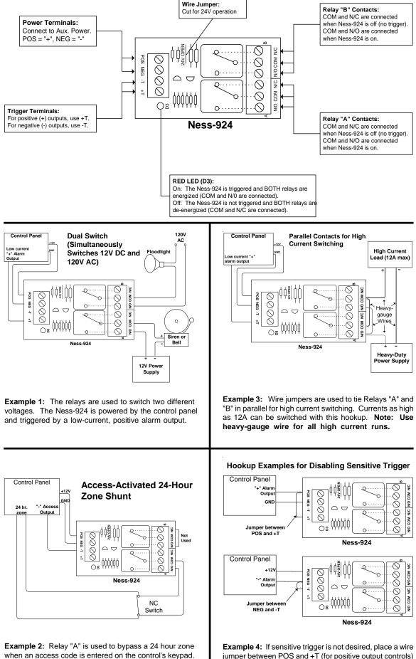
The "-" Access Output is connected to -T on the Ness-924.
